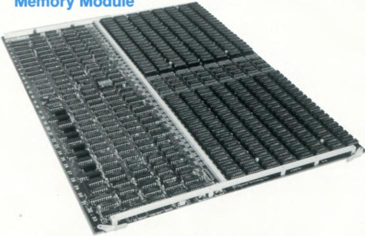
The MegaRam memory module is a semiconductor module employing 256Kx1 dynamic MOS integrated circuits. The capacity of the module is 8,388,608 bytes which can be organized as 2,097,152 words of 32 bits per word or 4,194,304 words of 16 bits per word. The module contains a comprehensive error detection and correction (ECC) capability which allows single bit errors to be corrected automatically.
