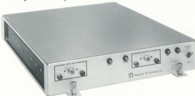
The battery back-up option consists of an optional power supply assembly which replaces the standard assembly inside the MegaRam chassis. This optional supply contains a battery pack capable of supporting a full 40 megabyte capacity MegaRam system for approximately 10 minutes. Additional support time can be obtained by adding external batteries.
